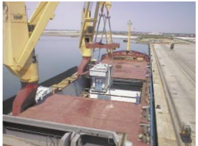
221 TONS TRANSFORMER BEING LOADED ON BOARD BBC-FRISIA IN FOS.
